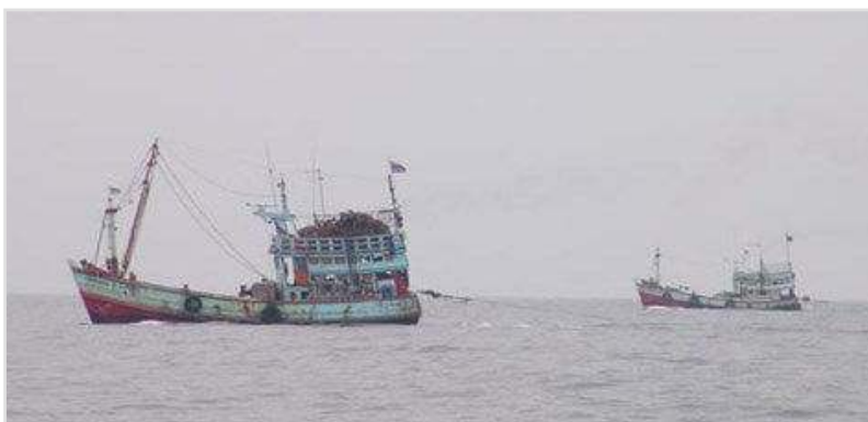
Two pair trawlers fish in tandem at a consistent distance and speed, dragging a net suspended between the two boats.
